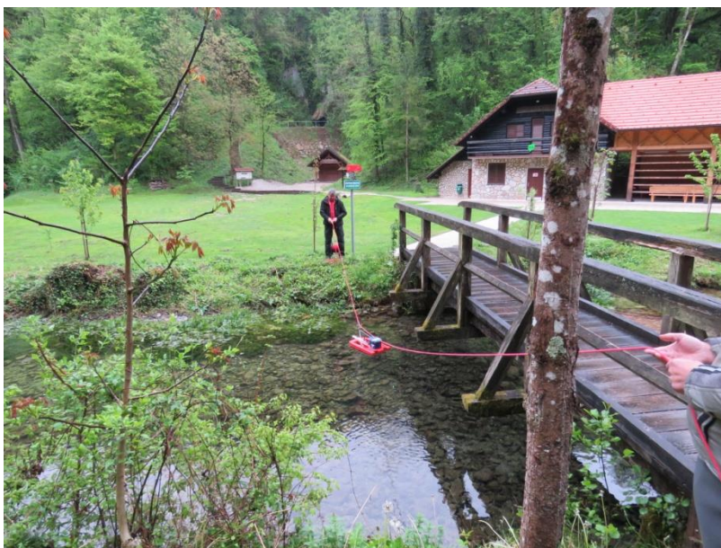
Slika 3. Meritev pretoka na območju izvira Studene v Globočicah 18. aprila 2017 (Foto: arhiv ARSO) Figure 3. Discharge measurement of Studena spring in Globočice on 18 th of April 2017 (Photo: ARSO archive)
