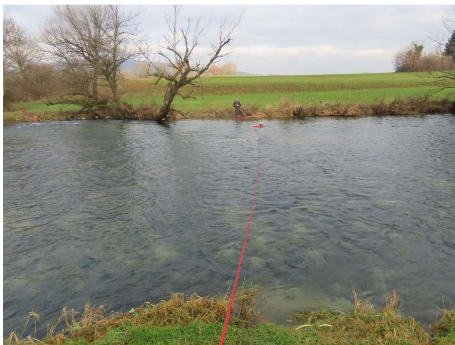
Slika 1. Meritve pretoka Krke v njenem povirju na območju Podbukovja, 17. decembra 2020 (foto: arhiv ARSO) Figure 1. Krka river discharge measurement on 17 th of December 2020 at its headwaters in Podbukovje (photo: ARSO archive)
