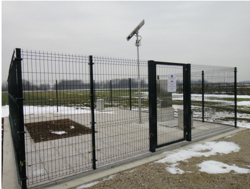
Slika 1. Merilno mesto za spremljanje gladine podzemne vode v Gančanih na Prekmurskem polju, 8 januar 2015 Figure 1. Measuring station for groundwater level observation in Gančani in Prekmursko polje aquifer, 8th of January 2015
