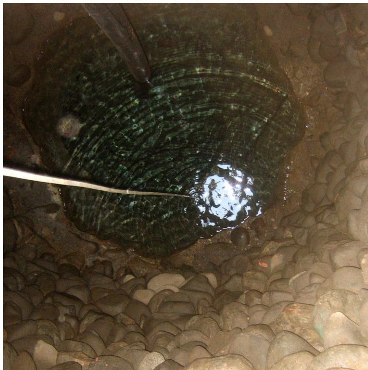
Slika 1. Meritev vodne gladine v gasilškem vodnjaku Latkova vas, dolina Bolske; julij 2011 (P. Souvent) Figure 1. Groundwater measurement in fire fountain in Latkova vas – Bolska valey; July 2011 (P. Souvent)
