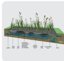
Figure 8: Schematic cross-section field constructed wetland ([www.limnos.si](http://www.limnos.si))
